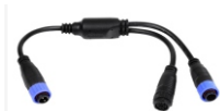
Item: AC-LEADIN-T336 DLP Lead in T connector cable at the first fixture of the daisy chain. It combines the power and signal into a 6-pin male cable. (3-pin male end for Power, 6-pin male end for data, and 6 pin female end to the fixture)
