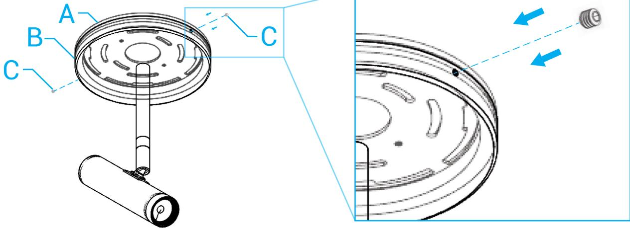
3.1) Secure Fixture (B) cover plate with the Ceiling Plate (A) by fastening the Set Screws (C).
