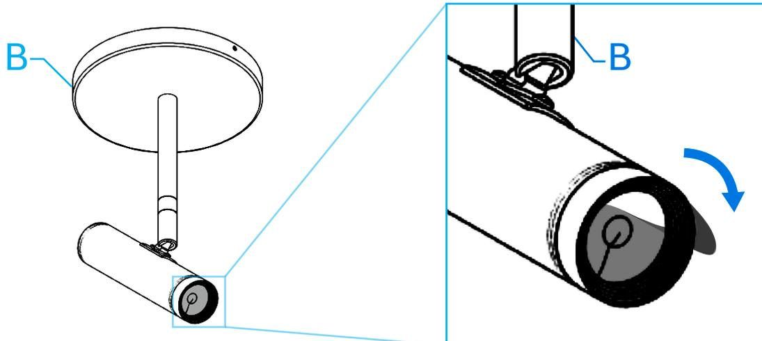
4.1) Remove the protective tape from the bottom light of the Fixture (A) prior to powering on.
