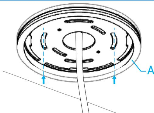
2.1) Proceed to secure Ceiling Plate (A) with fastenal screws. (Please note: Screws are not provided.)
