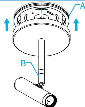
2.2) Align Fixture (B) cover plate with the Ceiling Plate (A).
