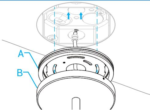
1.1) Feed the Fixture (B) cable wires through the Ceiling Plate (A), then connect cable wires with the Junction Box wires.
