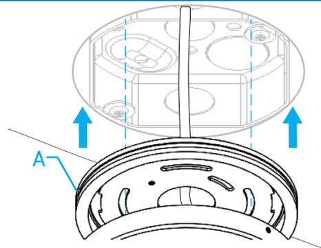
1.2) Align the Ceiling Plate (A) within the Junction Box.
